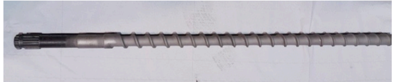
Extrusion screw: CarBoNiP™ coating + Teflon™
