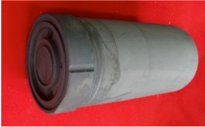
Plastic materials reinforced mould: CarBoNiP™ coating + Teflon™
